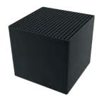
The dissociated recirculation - Box R allocates 9 to 10 Helsa charcoal cubes creating a system that enables up to 4000 parallel flow channels, capturing grease and odours very effectively. By separating the air in multitude of channels, this system also acts like silencer reducing the noise of the air flow.
