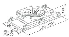
The SCL 360 hood is only installed on a false ceiling, for this the false ceiling must be able to support a weight of 30 kg.
