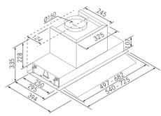
The Soul has flexible installation options, allowing for rear or standard (top) ducting:
