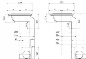
Motor box can be positioned to the front or the back to allow for full depth drawers.
