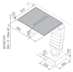
We need to leave a fix space of 40 mm from the wall to the edge of the hood and 50 mm to the cut out
