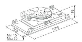
The Bright 360 hood is only installed on a false ceiling, for this the false ceiling must be able to support a weight of 30 kg.
