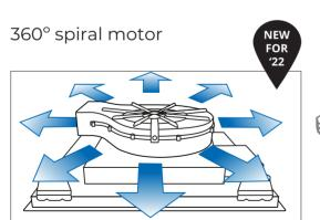
The new 360° spiral motor is now more efficient than ever. The design allows the extraction ducts to be installed in any direction, permitting ease of installation even in wall kitchens, where the ceiling hood is installed closer to the wall. With new aerodynamics, it uses less force to get better results by providing higher performance with lower energy consumption and maintaining a very low sound level.
