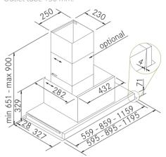
Optional top tube not suitable for cylindrical plasma and FC-Plus
