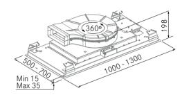
The Nitro 360 hood can only to be installed to a false ceiling, for which the ceiling must be constructed to withstand a weight of 30kg.
